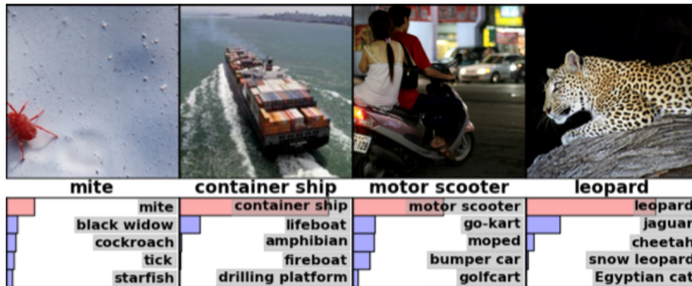
Figure 4: Object Recognition using a CNN trained with ImageNet data (from Krizhevsky, Sutskever, and G. E. Hinton 2012)
